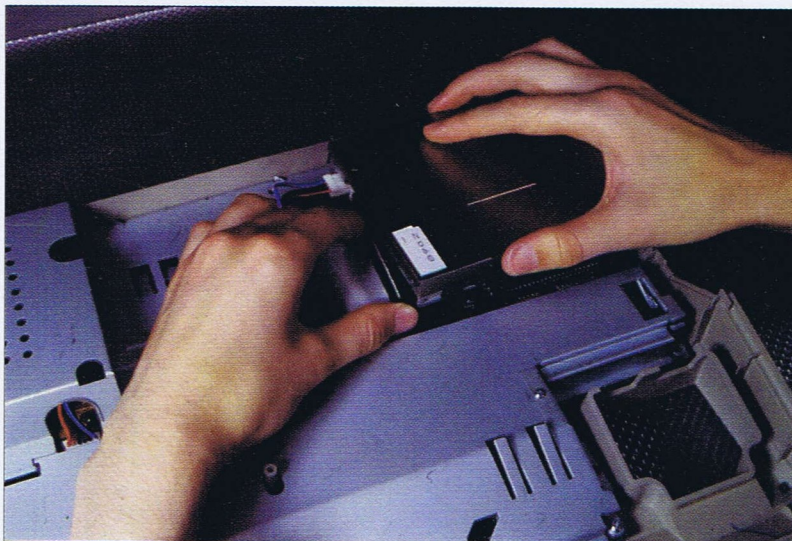
Once the ST is opened, removing the disk drive is simply a matter of unscrewing three mounting screws, then unplugging a power and data lead
